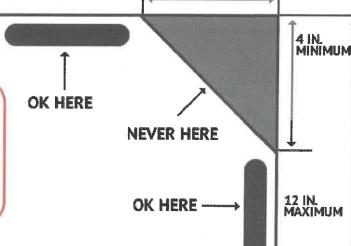
**NOTE:** Measurements shown are to the closest edge of the detector.
